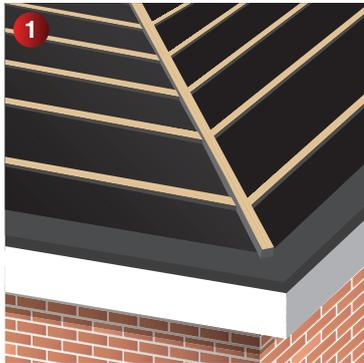
**1** Lay underlay as normal ensuring that the underlay overlaps the other side by 150mm min, and install tiling battens to the hip rafter or to noggins nailed to the hip rafter.
