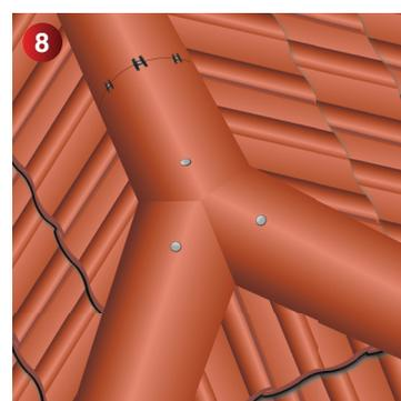
**8** Cut the tiles to form a neat mitre junction at the ridge hip junction. Drill a hole near the mitre and mechanically fix each tile with a screw to the batten. Seal openings in the cut tiles with a roofing grade mastic sealants.
