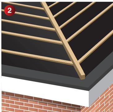
**2** Build up the hip batten on the hip rafter, to a height such that the hip tray overlaps the tiles on both sides and secure with nails.
