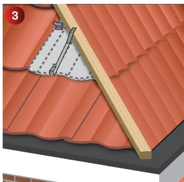
**3** Lay tiles as normal, ensure neatly cut tiles along the hip battens are no more than 30mm from the battens, and secured using the long and short hip clips provided. Nail the long hip clip to the batten through the holes provided, and then slide the cut tile into the clip below. Clip the short hip clip to the top end of the cut tile, attaching it to the adjoining tile at the interlock.
