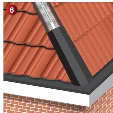
**6** Lay the hip trays centrally over the hip roll, overlapping the next tray by approximately 75mm and secure with nails.
