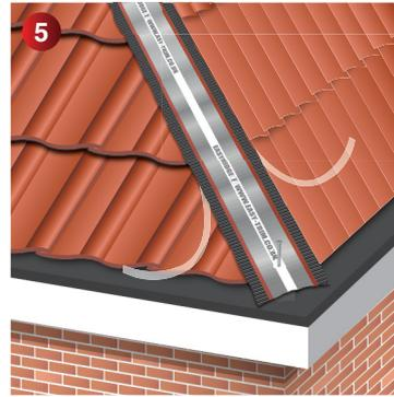
**5** Remove the release paper from the butyl adhesive strip on the underside of each edge of the roll, and firmly press onto the clean, dry tile on both sides (avoid crushing the corrugations). Ensure the rolls overlap at the hip abutment, and at the eaves carefully tuck back and stick behind the tiles
