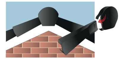
7 Continue this process up along the bargeboard along both sides until you reach the ridge. Insert a Ridge Cap, ensuring that the flexible flaps on the Ridge Cap contour around the outside of the Verge Unit. Fix the Ridge Cap to the ridge batten.
