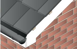
Lay tiles set flush with the battens. Remove existing mortar bedding in refurbishment project and install new tiling batten to the underside of the existing tiling batten.
