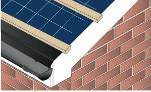
Install the tiling battens with a 30mm overhang, over the brick or barge board. Remove existing mortar bedding in refurbishment projects and install new tiling batten to the underside of the existing tiling batten.
