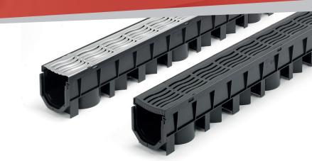
Channels are 1 metre in length with grates available in plastic or galvanised steel. They feature 3 vertical outlets for flexibility, as well as horizontal entry/outlet points which can be connected to either 100mm or 110mm pipes. A complete range of accessories creates a full, flexible system which is easy to install and maintain.
